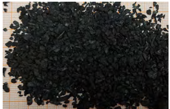
Figure 3. Biochar sample produced in the first gasification test campaign.
