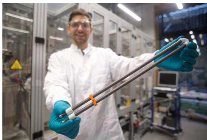
Figure 6. U-shaped oxygen transport membrane.
