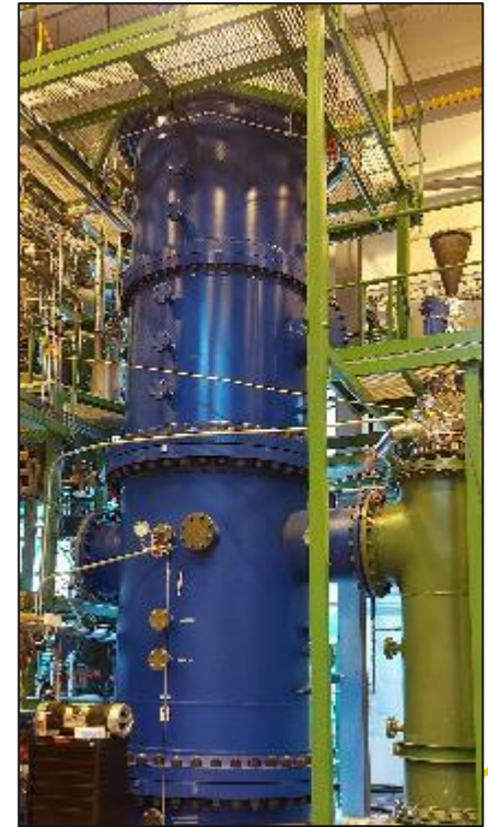
Pressurised fluidised-bed gasification pilot as the test platform (@ VTT Bioruukki in Espoo, Finland)
