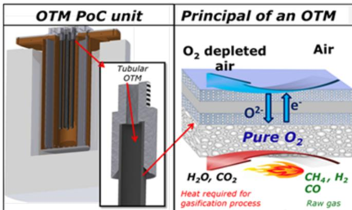
Figure 5. Operating principle of an oxygen transport membrane.
