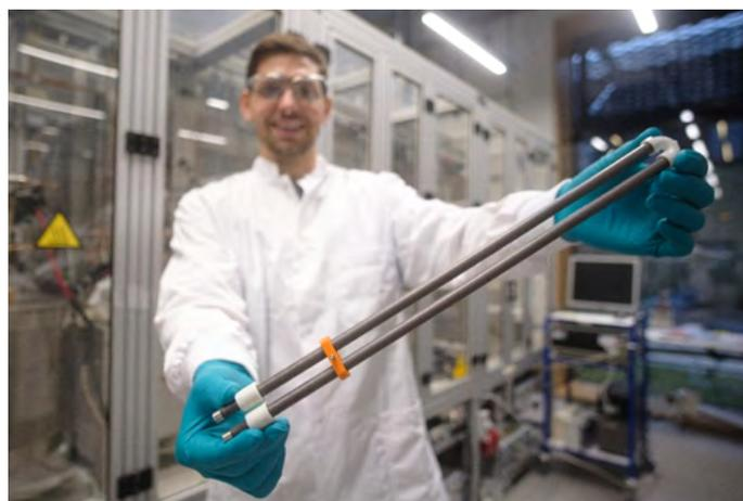
Figure 6. U-shaped oxygen transport membrane.
