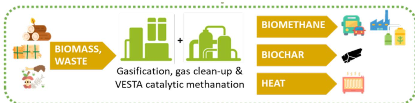
Figure 1. Schematic diagram of the FlexSNG process.
