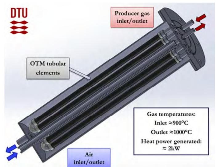
Figure 7. The core unit of the OTM reactor.
