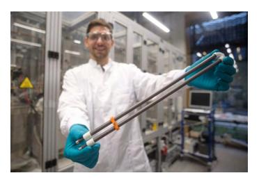
Figure 6. U-shaped oxygen transport membrane.
