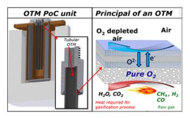
Figure 5. Operating principle of an oxygen transport membrane.
