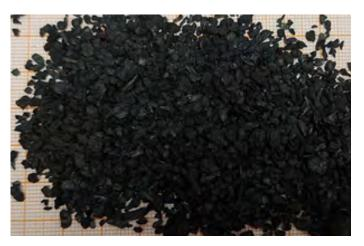
Figure 3. Biochar sample produced in the first gasification test campaign.
