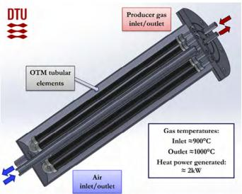
Figure 7. The core unit of the OTM reactor.
