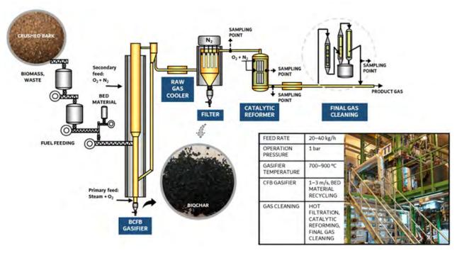
Figure 4. BCFB gasification pilot at VTT's Piloting Centre Bioruukki, Finland.
